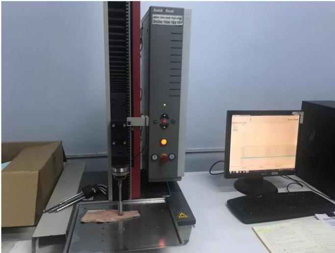
Picture 3. A Zwick/Roell 1.0 texture analyzer connected to a computer
