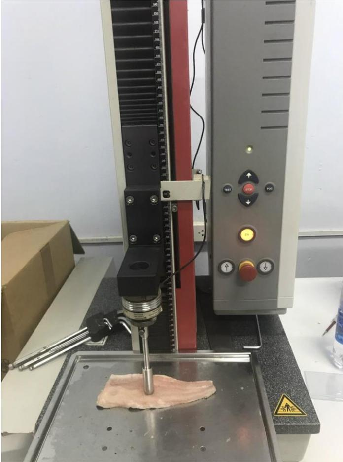
Picture 4. Measuring the hardness of a fish fillet of striped catfish (middle position)
